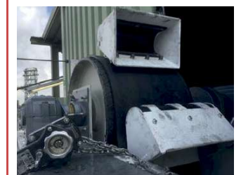
Shaft to drive pulley attachment by taper locking device
