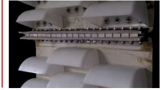
TECHNICAL SPECIFICATION - SUPER STARCO PLASTIC ELEVATOR BUCKET
