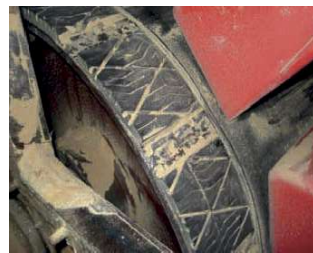
Close up of the Slide-Lag pulley lagging welded on the surface of the drive pulley
