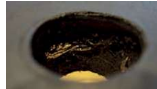
CNC drilled hole in Polysur® FERRO steel cord reinforced elevator belt. Dry process no water involved
