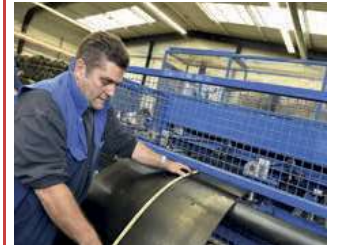
Polysur® EP textile reinforced rubber elevator belt provided with CNC punched elevator bucket bolt holes. Two rows of elevator buckets situated in staggered pattern on the elevator belt
