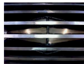
Wing pulley close up with the internal double cone showing
