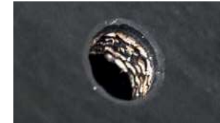
CNC punched elevator bolt hole in Polysur® EP textile reinforced rubber elevator belt
