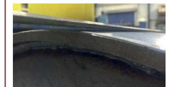
Close up of crowning on drive pulley surface
