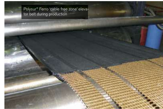
Polysur® Ferro SW-R/RE 'cable free zone' carcass
