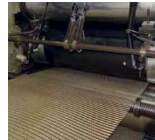
Polysur® Ferro SW-RE elevator belt during production
