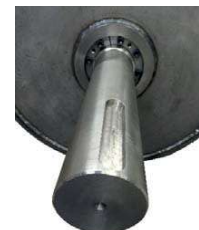
Shaft showing with 1 step rejuvenation and with keyway
