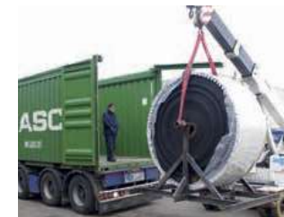
Loading a 8.2 tons Polysur® Ferro elevator belt with crane in a 20' ft. open top high cube container
