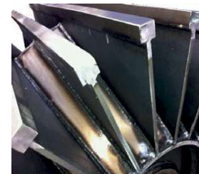
Close up of the wings that support the elevator belt
